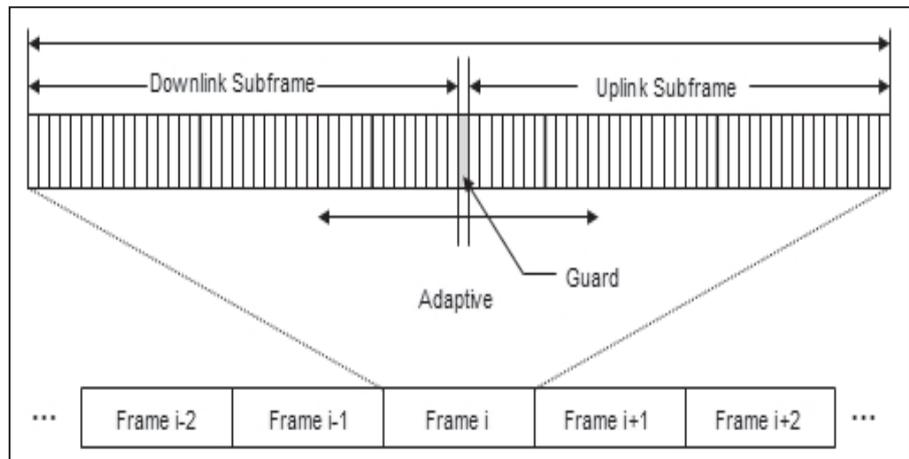
Figure 1. TDMA-frame structure
